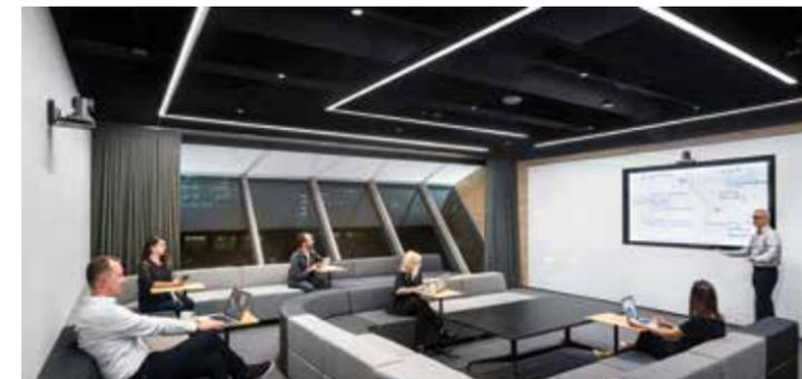
(both by Lumenwerx) provide bright, diffuse lighting for video conferencing, while small cylinder downlights (Gotham) offer focused lighting for dimmed video viewings. “The *downlights are arranged in a U-shaped pattern to relate to the seating configuration* below, and the row of linear wall washers illuminates the white board at the front of the room,” Klingensmith says.
