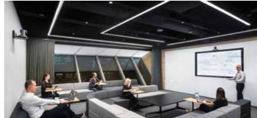
(both by Lumenwerx) provide bright, diffuse lighting for video conferencing, while small cylinder downlights (Gotham) offer focused lighting for dimmed video viewings. "The downlights are arranged in a U-shaped pattern to relate to the seating configuration below, and the row of linear wall washers illuminates the white board at the front of the room," Klingensmith says.
