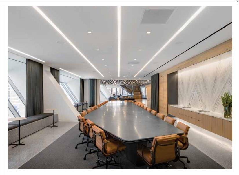
mployees can use a variety of spaces for meetings and events, including the board-room, where integrated accent lights and concealed slots form two major design elements. "The accent light has a 45-deg angled housing concealed along the bottom of the perimeter credenza to create a wash of light on the floor," Klingensmith says. "This 'toe kick' detail makes the credenza appear to float."
